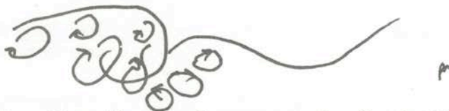
Fig. 3-15: Hypothetical movement of particle in broken wave.
