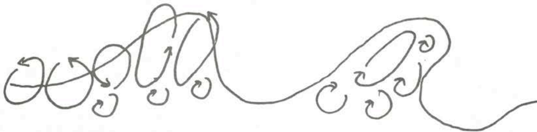
Fig. 3-14: Hypothetical movement of particle in breaking wave.
